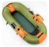
Insert floorboard after inflating safety chamber. Angled corners of board go nearest rod holder bases. Holes in board are not used with PF7.
