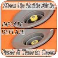
Press and turn stem counterclockwise so it can pop UP. When the stem is up, valve is closed and will hold air. To let air escape for deflation, press and turn stem clockwise until locked open.
