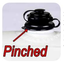
A common error is to pinch the retainer ring between the valve body and base. Trapping the ring breaks the air tight seal. If excess material covers the groove, the ring will go over if stretched slightly.
