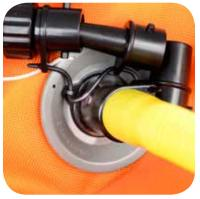
Inflate safety chamber first (front valve) with recessed valve adapter in hose. Push and turn adapter clockwise into valve opening. Pump air until chamber is almost full, but not firm. Twist hose counterclockwise and pull out. No air should escape. Replace cap in opening.
