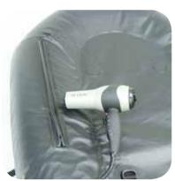
There are four tracking strips on the bottom of the boat which help to maintain course. The tracking strips are very flexible but if they become deformed, heat with a hairdryer until they return to their original shape (1-3 minutes).
