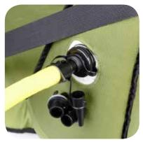
Push or screw valve adapter into valve. Inflate seat until comfortably firm. The back bladder can be fully inflated, or partially deflated to give more legroom.
