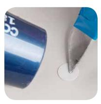
Apply patch to the boat. Smooth with finger or a smoothing tool such as a spoon, handle of a utility knife, or screwdriver. For best results, heat patch with a hair dryer 10-20 seconds and smooth with tool.
